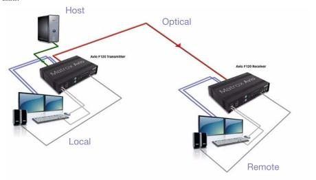
■ Host – Connections between the host system and the transmitter unit. The computer is the only host device. You must connect the video output of your graphics card to the video in connectors on your transmitter unit and your computer to the main USB connector on your transmitter unit. To use the sound connectors at the front of your transmitter or receiver units, you also need to connect the sound input and output of your computer to the transmitter unit.
