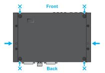
■ Use a hand screwdriver to carefully tighten each screw. Make sure not to overtighten the screws.
